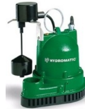
SKU V-A1 Cast iron, 115V, 1/3 HP submersible sump pump 1 Phase with 10' cord
